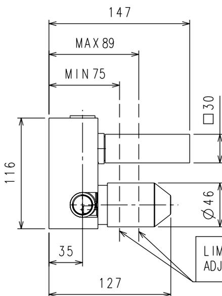
LIMITI PER LA SUPERFICIE FINITA DELLE PIASTRELLE
